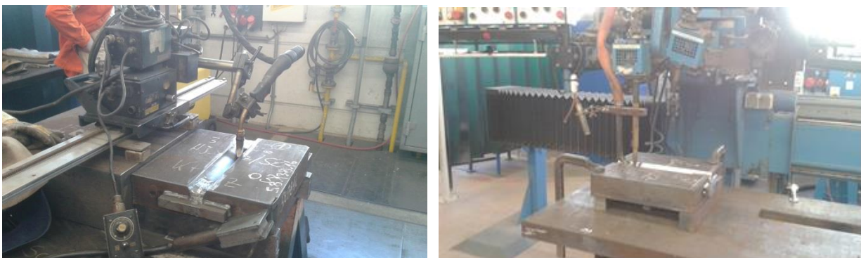
Figure 3: GMAW and SAW welding of Tekken test specimen
